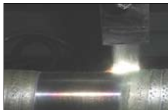
Cladding with diodelaser.
