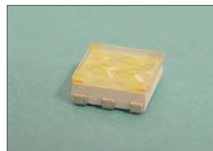
FIGURE 2. In wafer-scale UV embossing (REEMO®) of micro-optic components, the glass wafer with the UV-embossed microstructure is subsequently diced to produce individual components, which are packaged as required for an application. Generally, the size of the diced components is similar to that of small electronic components. This means that standard packaging can be used, such as a common tape and reel Assembly with, e.g., LED gives very small and thin module solutions.
