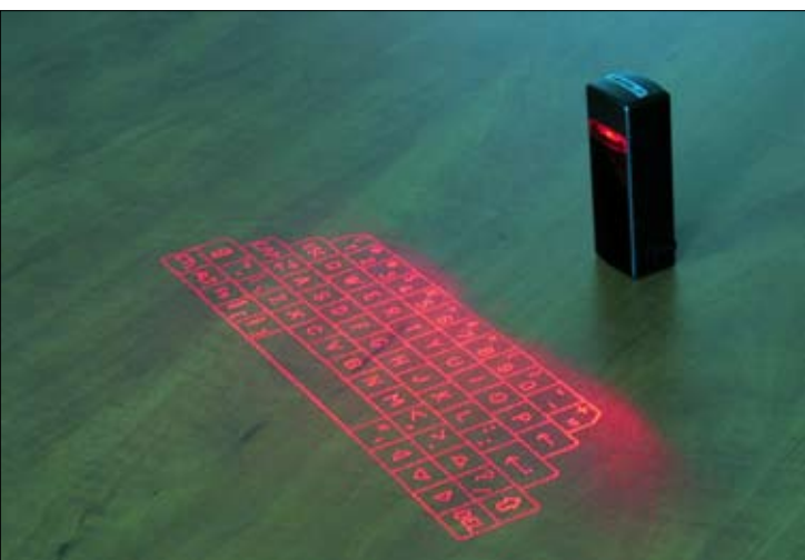
FIGURE 1. A diffractive optical element (DOE) is used as a pattern generator for a virtual laser keyboard in personal data assistants (PDAs) and mobile phones. The replicated DOE projects a visible keyboard pattern that serves as a guide for the user's fingers. Finger position is detected by a plane of infrared light and a CMOS sensor module.
